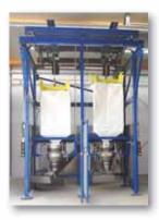
Big Bag Handling System with 2 JDN (Air Hoists) PROFi 2 Ti in Motor Trolley for operation in Zone 1. Important in this case was that the PROFis are suitable for oil-free operation.
